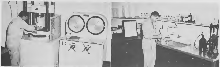
THE LARGEST and most imposing piece of equipment in the new Laboratory of the Equipment Inspection Group is the compression and tensile testing machine, above. Raymond Peterson adjusts sample to be tested, and, right, experiments with the acids used to identify materials and their structure. The new EIG lab is located in the main shops on the north side of the metal trades area.
